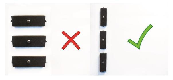
The minimum diameter of a concave or convex surface, as for example a pipe, is 1500mm. Smaller diameters can result in the magnet surface not getting fully in contact with the wall and greatly reduce its force.
